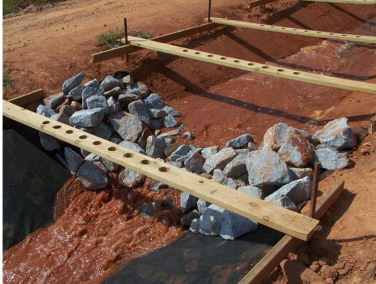
Figure 3.103 Test Setup for Ditch Check performance Evaluations (TRI Erosion Test 2019)
