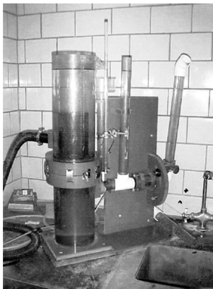
Figure 3.85 Constant Head and Falling Head Apparatus (ASTM D4491 2017c).
