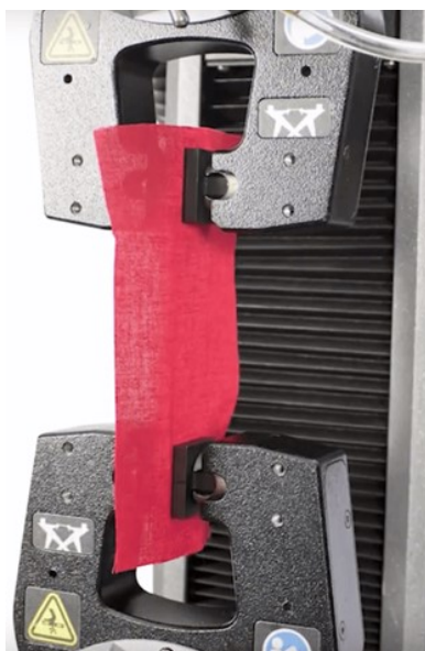
Figure 3.92 Woven Textile Fabric during Testing (Instron 2017).
