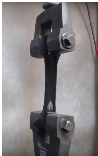
Figure 3.89 Elongation of Nonwoven Geotextile during Testing (Geosynthetic Institute 2018b).
