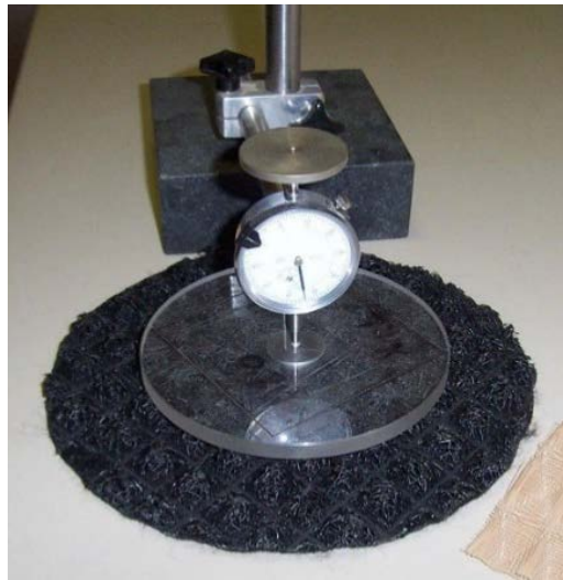
Figure 3.97 Thickness Measuring Equipment and a TRM (Geosynthetic Institute 2018f)
