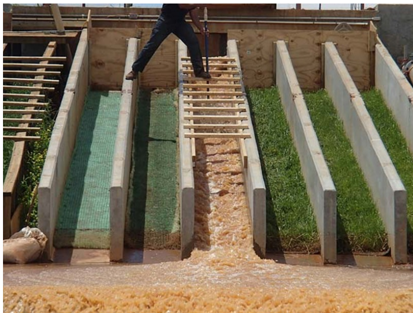
Figure 3.96 Full Scale Test Setup for RECPs (TRI Erosion Test 2019).
