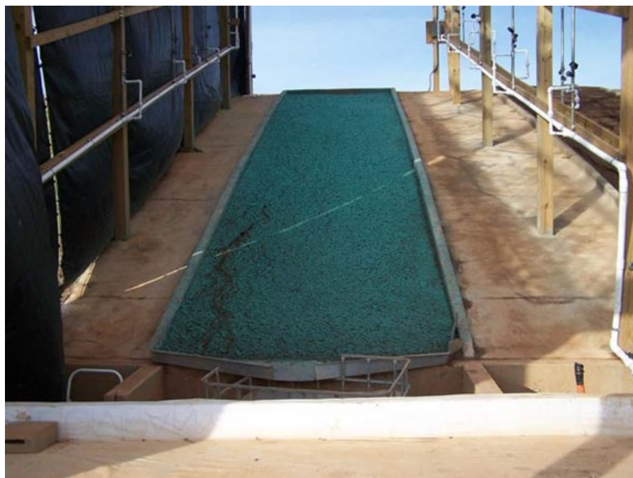
Figure 3.95 Test Setup for Testing RECPs (TRI Erosion Test 2019).
