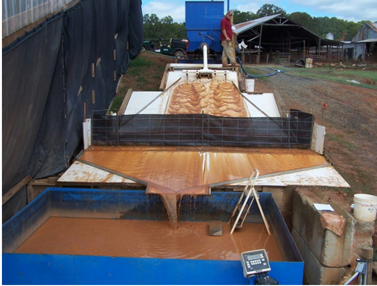
Figure 3.104 Testing Setup for SRDs Evaluation (TRI Erosion Test 2019)
