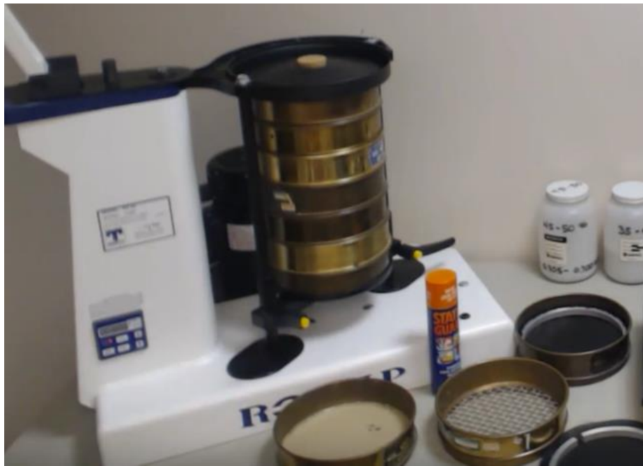
Figure 3.90 Ro-Tap Sieve Shaker Balance and Sieve (Geosynthetic Institute 2018c).
