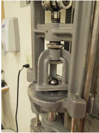
Figure 3.83 Ball Burst Arrangement (ASTM D3787 2016a).
