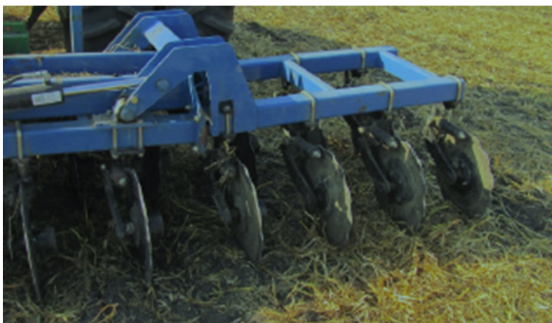
Figure 3.9 Dry Mulch Anchoring Process (Iowa DOT 2017).
