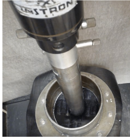
Figure 3.94 Geotextile Under 1.9 Inches Probe in Testing (Geosynthetic Institute 2018e).
